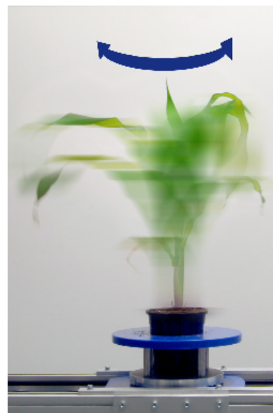
Lift-turtable for imaging
