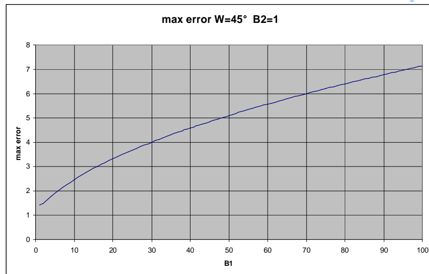
Figure 4: Dependency of maximum error for 45° from the ratio between B1 and B2 (here B 2 = 1).
